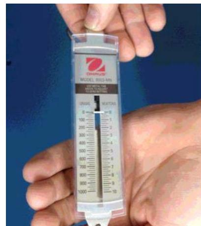
**Figure 3.** Zeroing the scale
