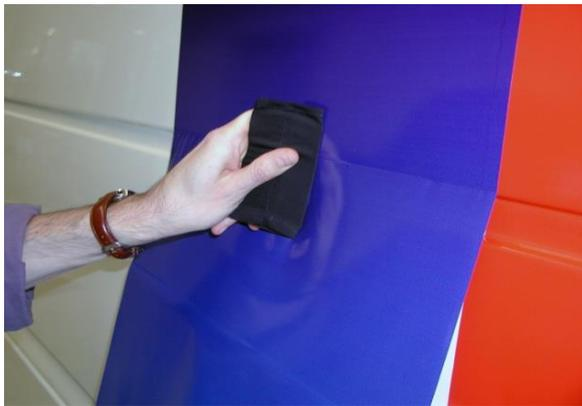
**Post-Heating** Ensure that no air bubbles are left trapped between the substrate and the film by re-heating the film in the recessed areas and corrugations with a hot air gun. By doing this, overlooked air bubbles can be detected. Air bubbles between the film and the substrate must be removed with the air release tool.
